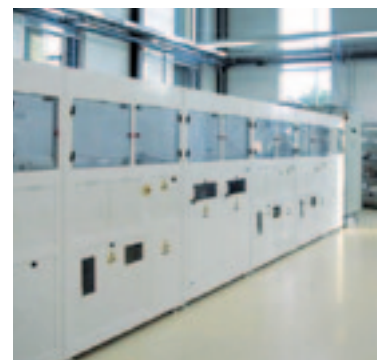
Wetbench made of SIMONA® PVC-C CORZAN FM 4910 G2
