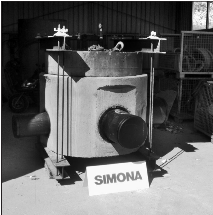
Successful leak test in accordance with DIN V 4034-1, monitored by the official Material Testing Institute (MPA) Darmstadt.
