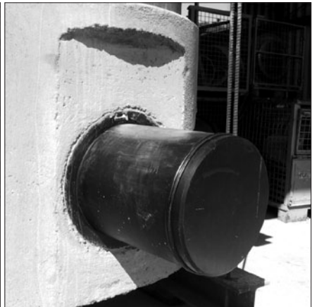
Successful leak test in accordance with DIN V 4034-1, monitored by the official Material Testing Institute (MPA) Darmstadt.
