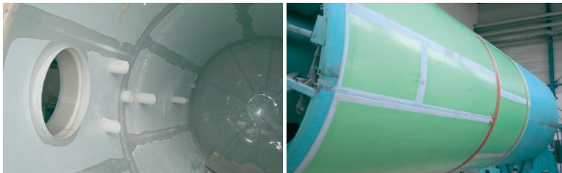
GFRP composite tanks are six metres long and 2.4 metres in diameter. The SIMONA® PVDF-GK sheets are clearly visible in the construction phase (below).
