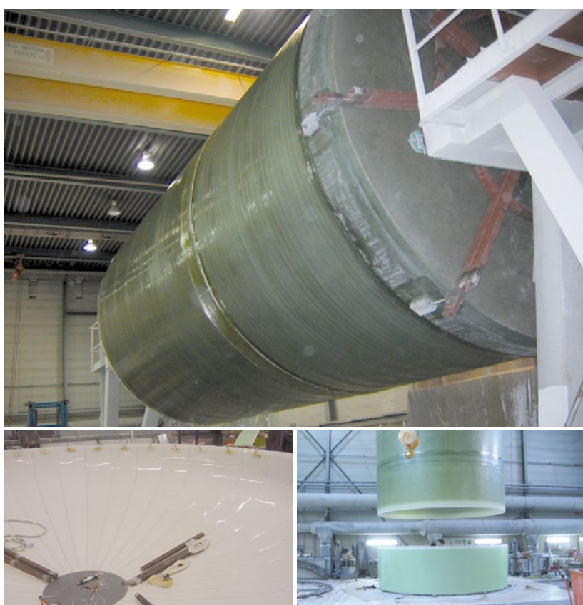
The GRP composite tanks are eleven metres high and five metres in diameter.
