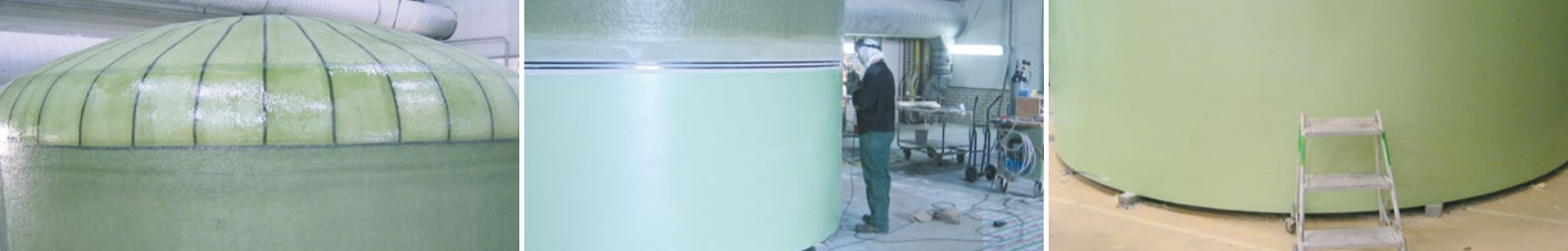
From left to right: Tank cover, manufacture of the cylindrical section, tank base
