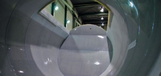
From left to right: View into the lower pipe sections with gas inlet, transport of the SIMONA® E-CTFE-GK/GRP composite pipe sections, SIMONA® E-CTFE-GK/GRP/steel ready for transport
