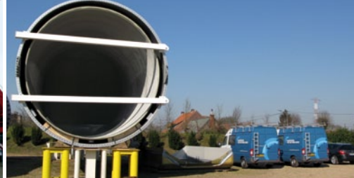
From left to right: View into the lower pipe sections with gas inlet, transport of the SIMONA® E-CTFE-GK/GRP composite pipe sections, SIMONA® E-CTFE-GK/GRP/steel ready for transport
