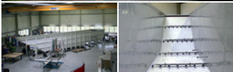
Above: Steel bath being loaded. Below: Internal lining with SIMONA® PP-DWU AlphaPlus. Steel bath with SIMONA® PP-DWU AlphaPlus inliner.
