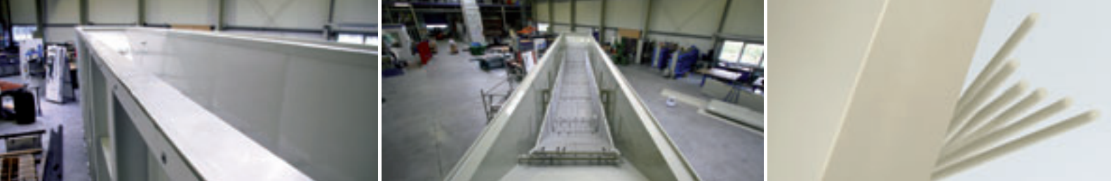
Pictures from left to right: Steel bath with SIMONA® PP-DWU AlphaPlus inliner, lined steel bath with collection basket, SIMONA® PP-DWU AlphaPlus sheet with welding rods.
