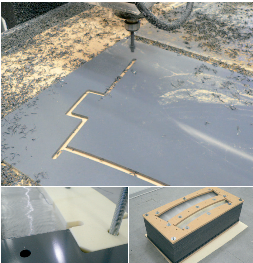
Above: milling out the individual formwork elements from SIMONA® PVC-CAW. Bottom left: building up the formwork with polyurethane separating strips and optical fibre mats. Bottom right: the finished formwork system.
