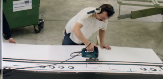
f.l.t.r.: Applying digital printing foil and black self-adhesive film to SIMONA® SIMOPOR-LIGHT Sheets; cutting of the individual elements; finished stage design
