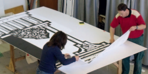
f.l.t.r.: Applying digital printing foil and black self-adhesive film to SIMONA® SIMOPOR-LIGHT Sheets; cutting of the individual elements; finished stage design
