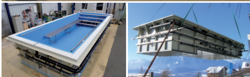
Top: outdoor whirlpool in operation; bottom left: construction and completion at Allplast AG; bottom right: transport by mobile crane
