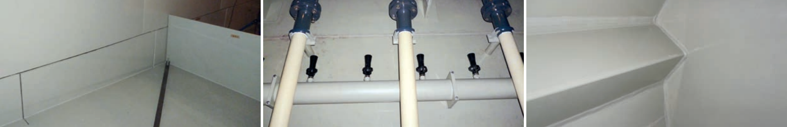
From left to right: Lining with SIMONA® PP AlphaPlus® Sheets; nozzle pipes comprising SIMONA® PP AlphaPlus® Pipes; safe welded connections with SIMONA® PP AlphaPlus® Welding Rods
