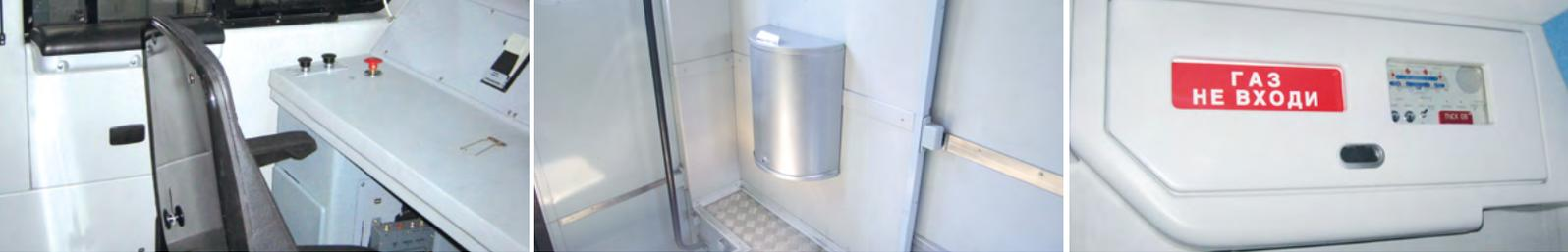
SIMONA® PVC-CAW-FR sheets in situ: wall and surface coverings as well as cover elements in the locomotive and around the entrance to a carriage
