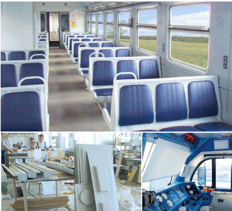
Top: carriages cladded inside with SIMONA® PVC-CAW-FR sheets; bottom left: manufacturing the coverings; bottom right: wall elements and dashboard in the driver's cab
