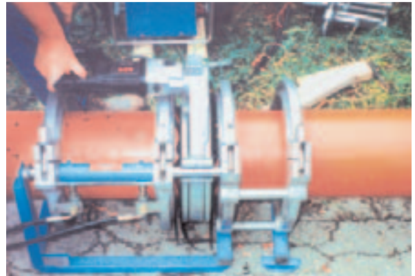
Preparing the pipes for heating element butt welding by planing the end faces
