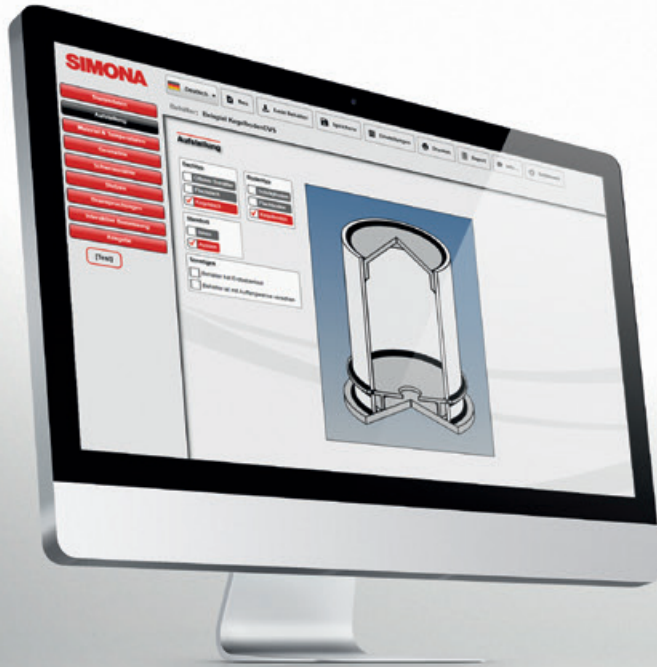
Cylindrical tank calculation – all shapes of roof and base components (as per DVS) can be calculated by the program.
