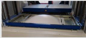
4. Forming process (here: vacuum forming; other forming methods possible)
