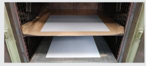
2. Heating to around 200°C (here: infrared heating; other heating methods possible)
